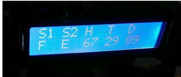
Figure 6. LCD display showing slot1 filled and slot2 empty
