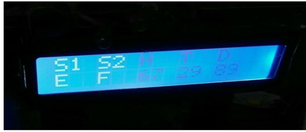
Figure 5. LCD display showing slot1 empty and slot2 filled
