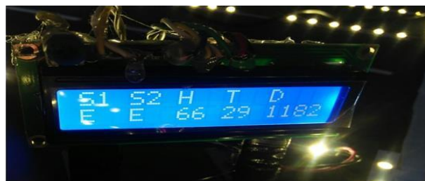
Figure 4. LCD Display Showing Both the Slots are empty
