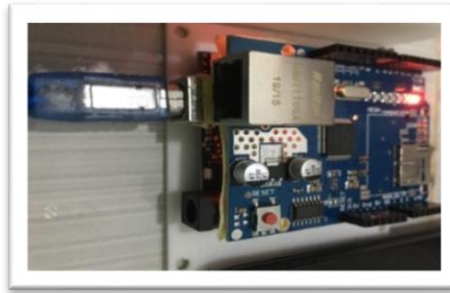
Figure 6. Arduino Uno and Lan Shield circuit
