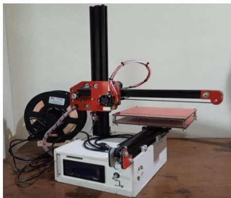
Figure 8. Final result of the Cartesian 3D Printer
