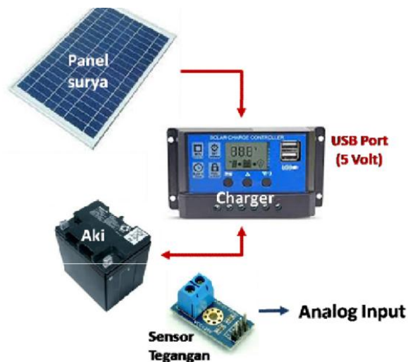
Figure 7. Portable power supply equipped with battery voltage sensor
