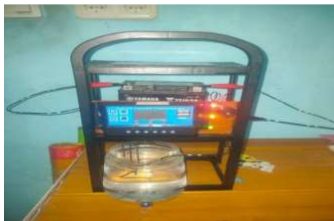
Figure 4. Water Level Detection Device Prototype Testing Process
