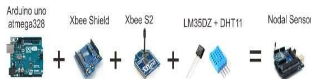
Figure 6. Nodal Sensor Device Components
