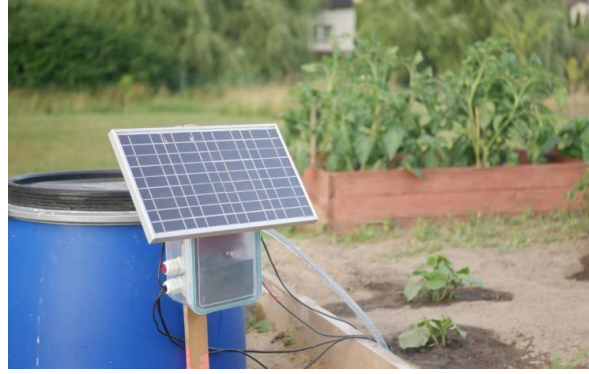
Figure 3. Electrical System with Solar Panel
