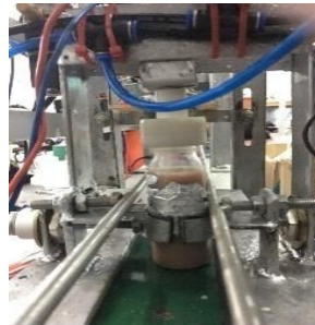
Figure 6. Bottles Detected on Capping Stations.
