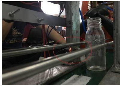
Figure 4. Bottles Detected at Filling stations.
