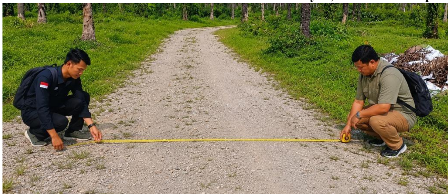
Figure 3. Road Width Measurement
