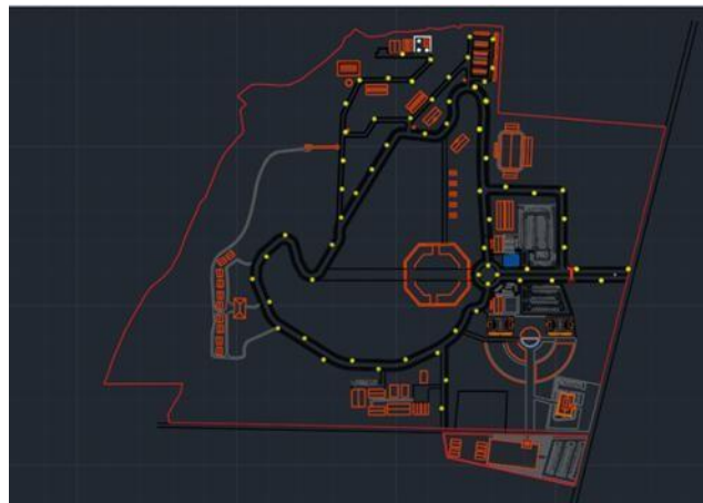
Figure 6. Determining the light point using AutoCAD software
