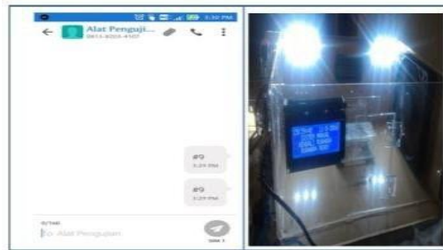
Figure 6. Test Results for Keyword #9 Turning on Electricity
