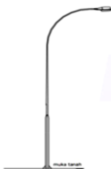
Figure 1. Single Arm Light Pole Source: BSN
