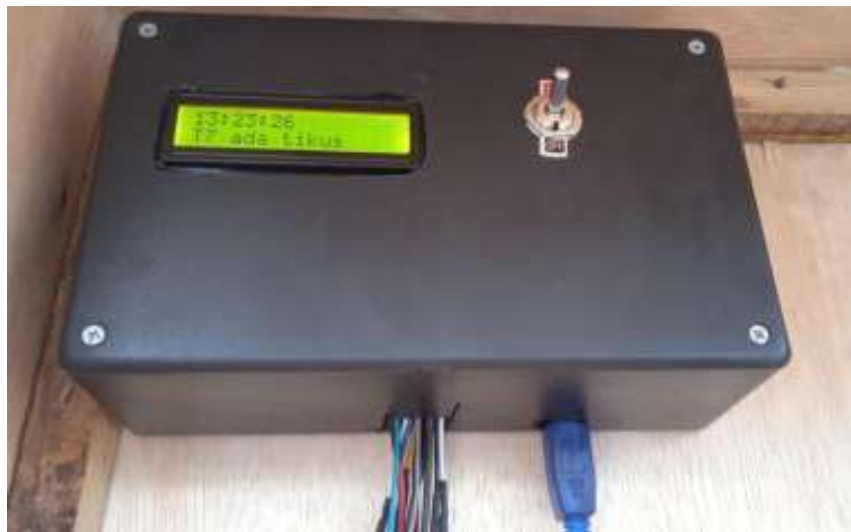
Figure 7. Pest Control System LCD Display
