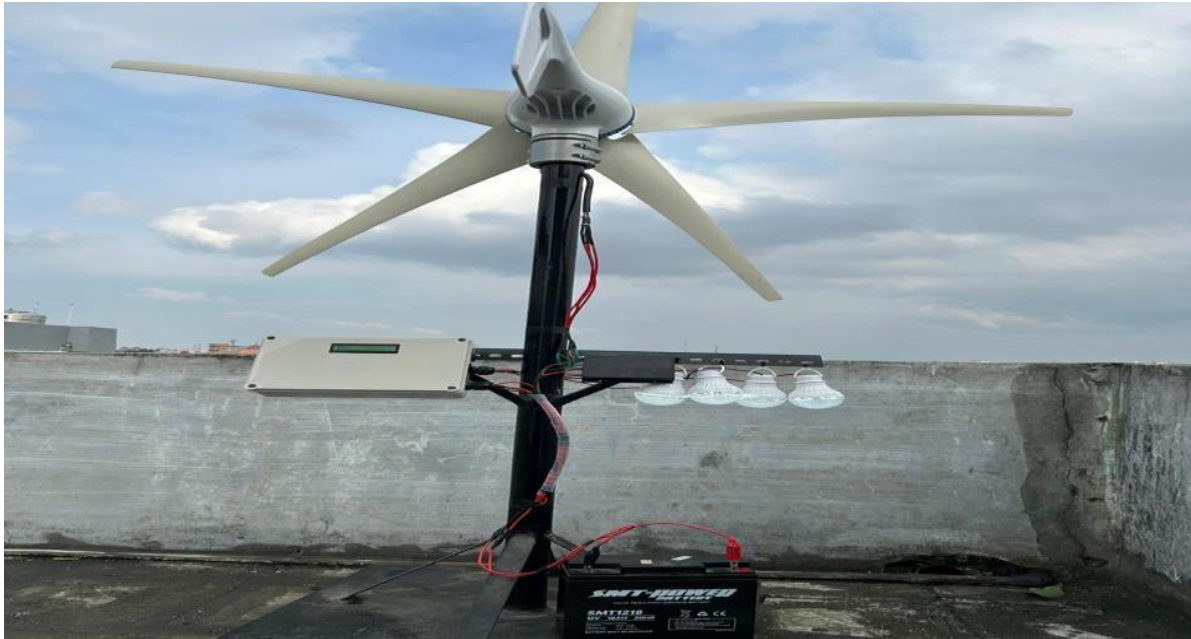
Figure 6. Prototype Design Results for IoT Monitoring of Wind Turbine Electric Power
