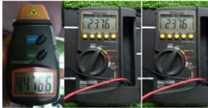
Figure 4. Results of rpm/V/A testing without load
