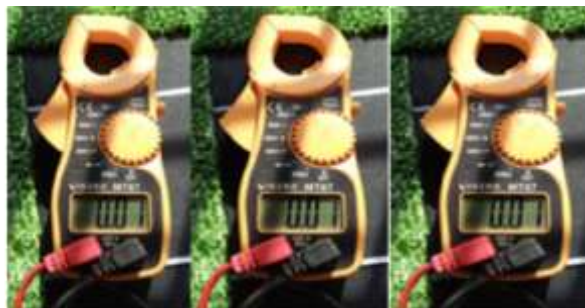
Figure 7. Results of the rpm/V/A test with a 10-Watt lamp load
