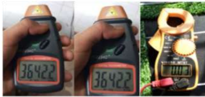
Figure 6. Results of rpm/V/A testing with a 7 Watt lamp load
