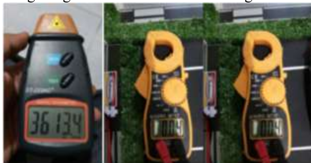
Figure 8. Results of the rpm/V/A test with a 12-watt lamp load
