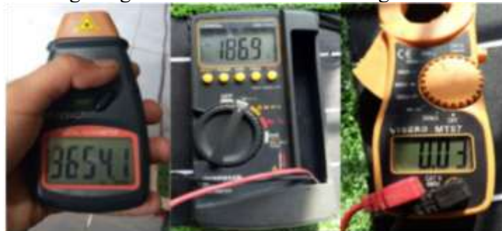
Figure 5. Results of rpm/V/A testing with a 2 Watt lamp load
