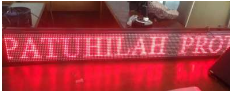
Figure 10: shows the text display results of the 2 tests on the P10 LED module, which is text. PATUHILAH PROTOKOL KESEHATAN
