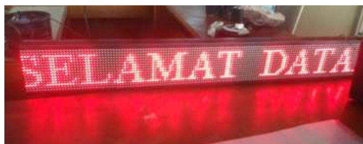
Figure 8 : shows the text display results of the first test on the P10 LED module, which is text. SELAMAT DATANG DI UNIVERSITAS PEMBANGUNAN PANCABUDI
