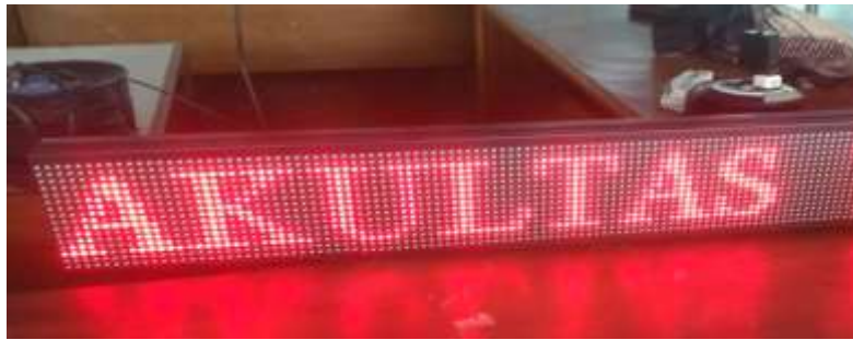
Figure 9: shows the text display results of 2 tests on the P10 LED module, which is text “FAKULTAS SAINS DAN TEKNOLOGI JURUSAN TEKNIK ELEKTRO”
